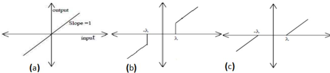
Figure (1) represents the threshold functions of linear (a), solid (b), and elastic (c).
